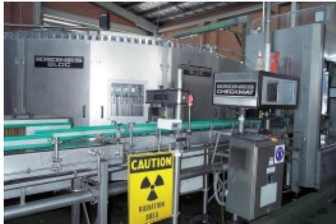
A bottle and can filling line is integrated with a UNIMETER XQL connected to a magneto transducer. From the digital reading, the bottle or can height is determined. This value is then used to set the height of the filling nozzle in the line. The UNIMETER XQL has two set points. The production line becomes more versatile and easier to operate, as it does not have to be totally reset for new batches of different height containers.
