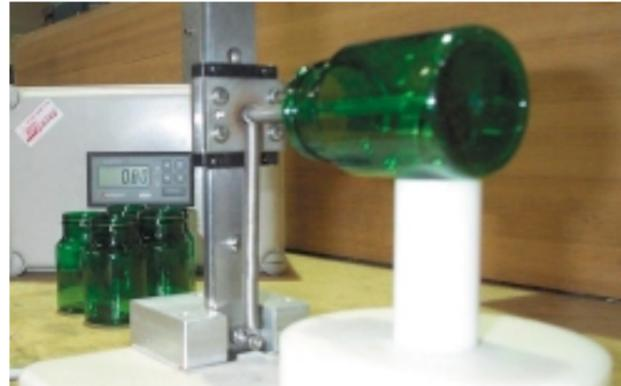
A producer of natural health products uses UNIMETER XQLs to measure and monitor both mould temperature and bottle thickness in the production of their bottles and containers. This provides an accurate and easy to operate measurement system. The UNIMETER XQL's USER OFFSET and TARE functions allow for quick and easy calibration.
