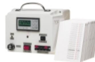
An advanced training exercise can be run to teach the programming and use of Special Functions such as set points and scaling. UniTrain is supplied with UniSoft V6.0 Software and a UniSoft Adapter (RS485 to RS232), so that instructors can demonstrate the use of a PC to capture and control data. Included are a set of 10 UNIMETER XQL manuals. UniTrain is housed in a robust, insulated carry-case, which can be connected directly to mains power.
